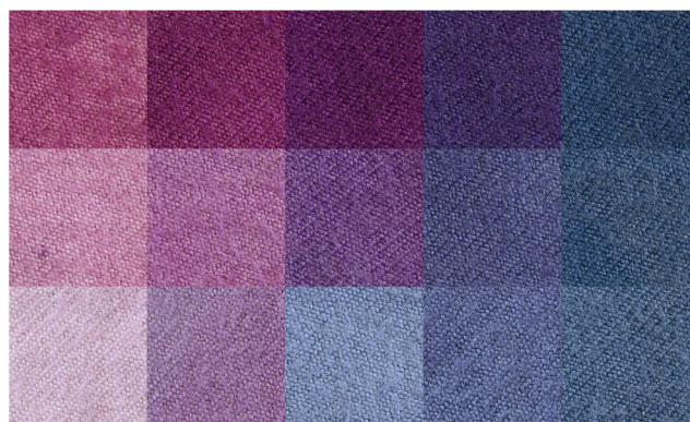
Fig. 2 Composite photograph of dyeings from five three-pass dyeing runs: (1st–5th columns) DBI, 1:1 DBI:MBI, MBI, 1:1 MBI:IND, IND; top-row squares are first-pass dyeings
