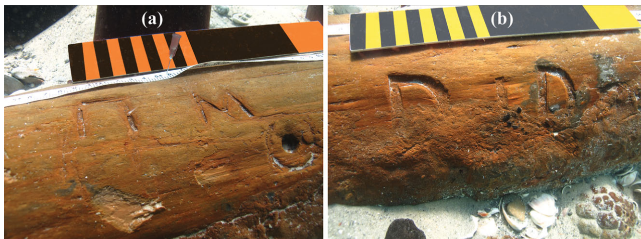
Figure 8. Stringer HL-12: a) incised Greek letters Pi and Mu; and b) unidentified markings (Photos: A. Yurman).
