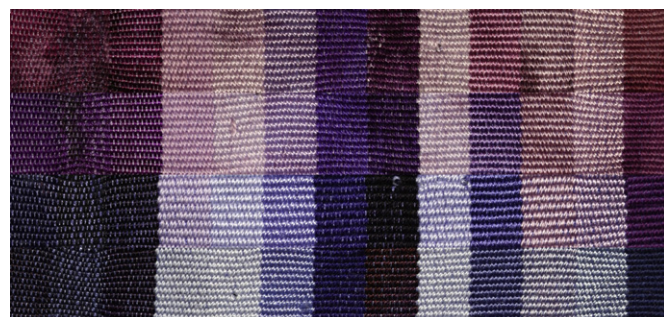
Fig. 8. Thermochromicity of multi-fabric strips dyed with DBI and MBI. Top to bottom: DBI heated, DBI unheated, MBI unheated, MBI heated. See Fig. 3 for fabric identities.
