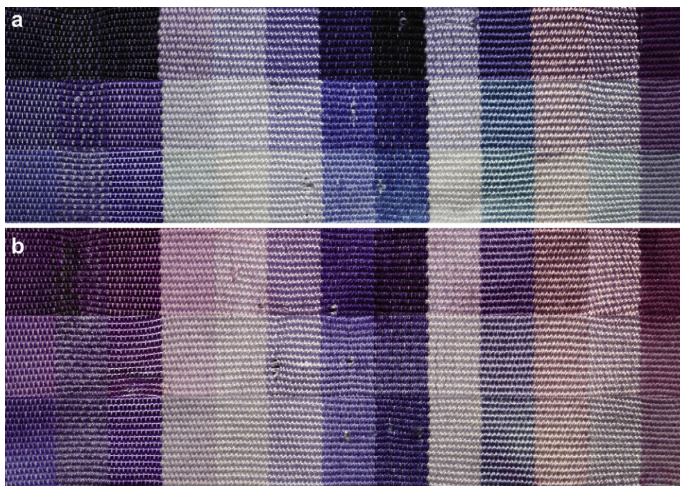
Fig. 4. Three-pass dyeings with (a) MBI (t to b: 1st, 2nd, 3rd pass); (b) DBI (t to b: 1st, 2nd, 3rd pass). See Fig. 3 for fabric identity.
