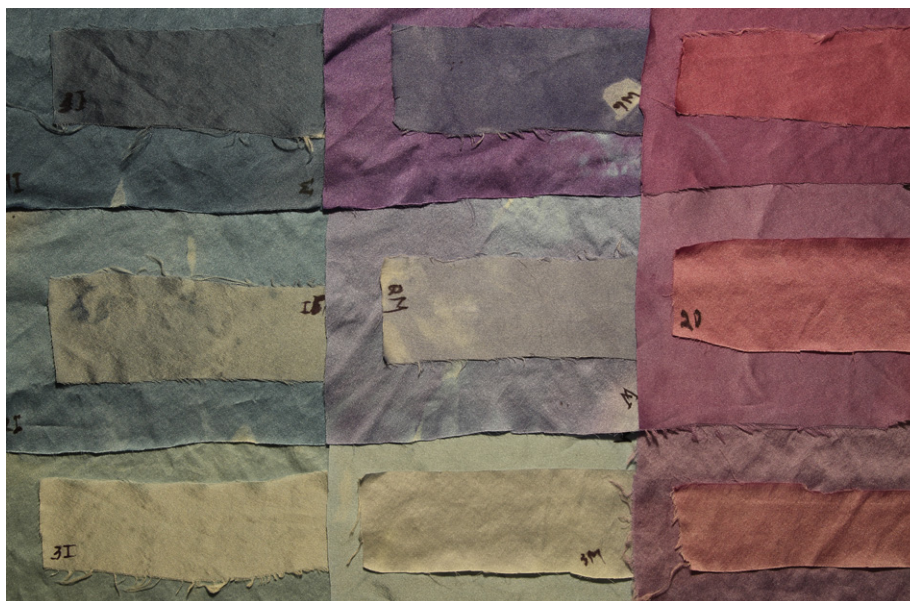
Fig. 6. Three-pass silk dyeing with indigo (left column), MBI, (middle column), and DBI (right column). Top to bottom: 1st, 2nd, 3rd passes; insets are heated.
